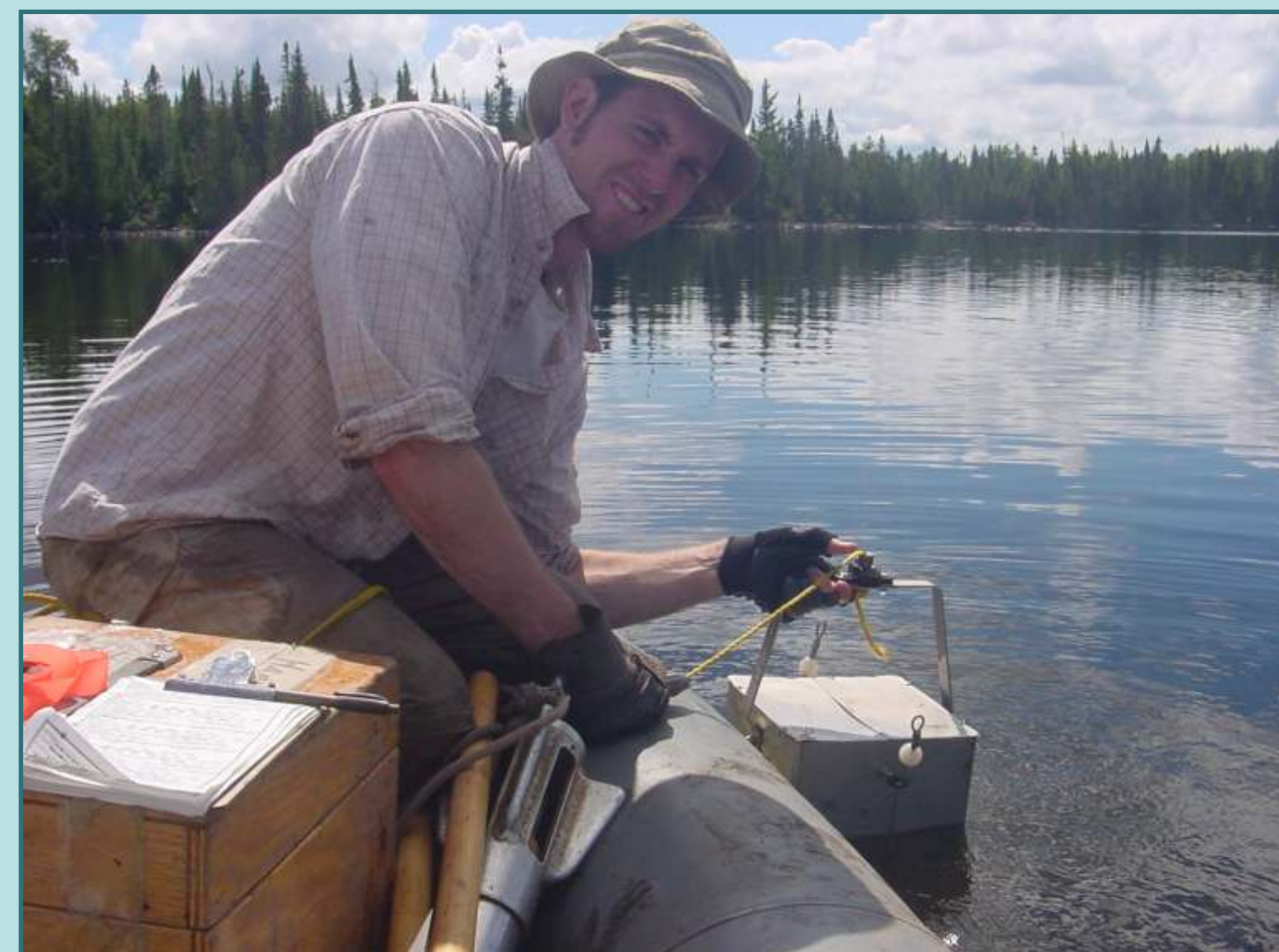
Photo 5. Ekman dredge breaking surface with lake sediment sampler.
