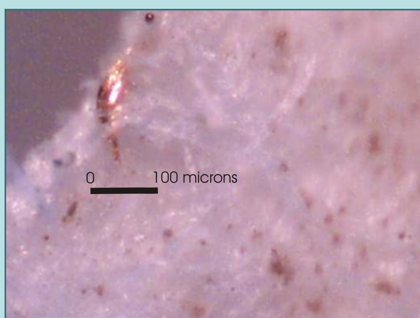
Photo 1. This image, obtained by binocular microscope, shows a gold grain (encased in glue) recovered from a 10 gram sample briquette analyzed by INAA and returned a Au value of 293 ppb.
