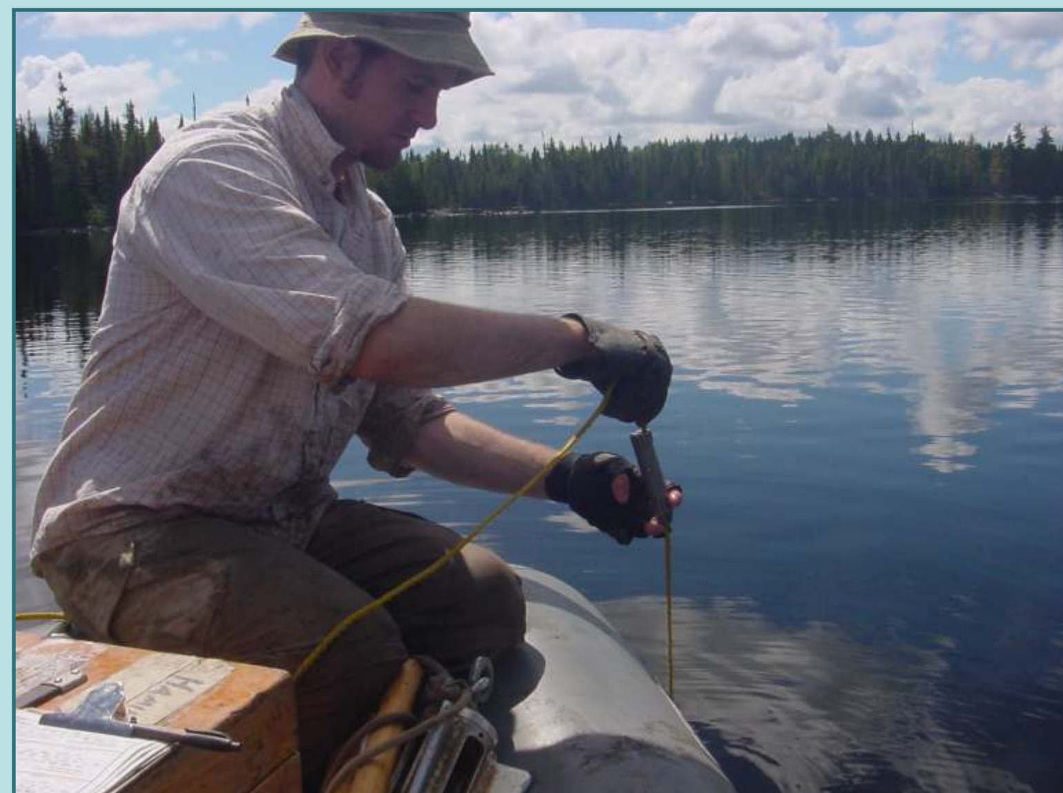
Photo 4. Lake sediment sampling with Ekman dredge. The messenger is about to be sent down to activate the jaws of the sampler.
