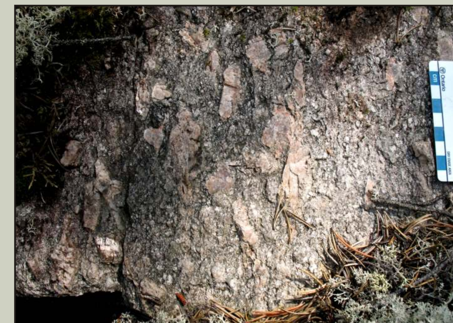
Photo 13. Cycle 2 is bound on the eastern side by this granite suite. It is generally well foliated with biotite and hornblende and is locally potassic feldspar megacrystic.
