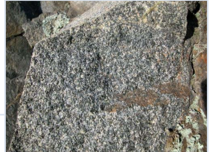
Close-up of intrusive diorite. Diorite has a distinctive "salt and pepper" appearance. Dark minerals are hornblende, light minerals are quartz and feldspar.
