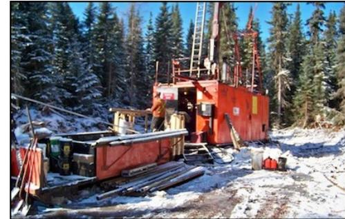
Diamond drilling uses a hollow bit whose surface contains low quality diamonds. It produces a long cylinder of rock referred to as a core.
