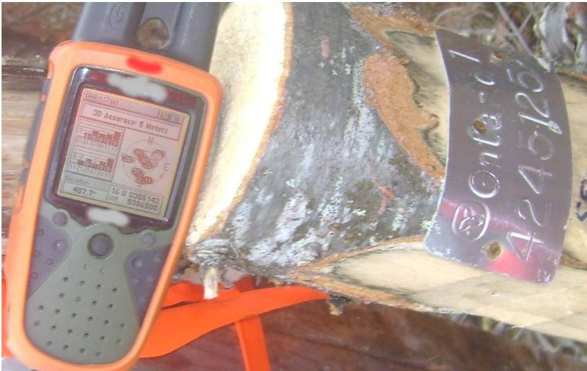
FIGURE 1: Example of a photograph of the claim post tag together with the satellite screen of the GPS receiver showing the GPS location coordinates.
